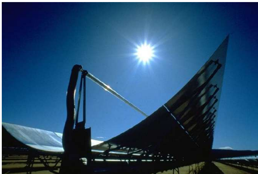
Figure 3.5: A solar trough, one of the most cost-effective and widely-deployed solar devices.
