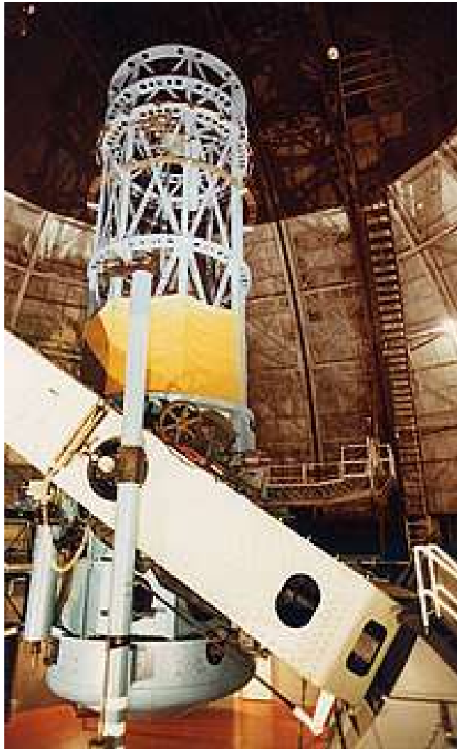
Figure 6.9: The 100-inch Hooker telescope at Mount Wilson Observatory that Hubble used to measure galaxy distances and a value for the rate of expansion of the universe.
