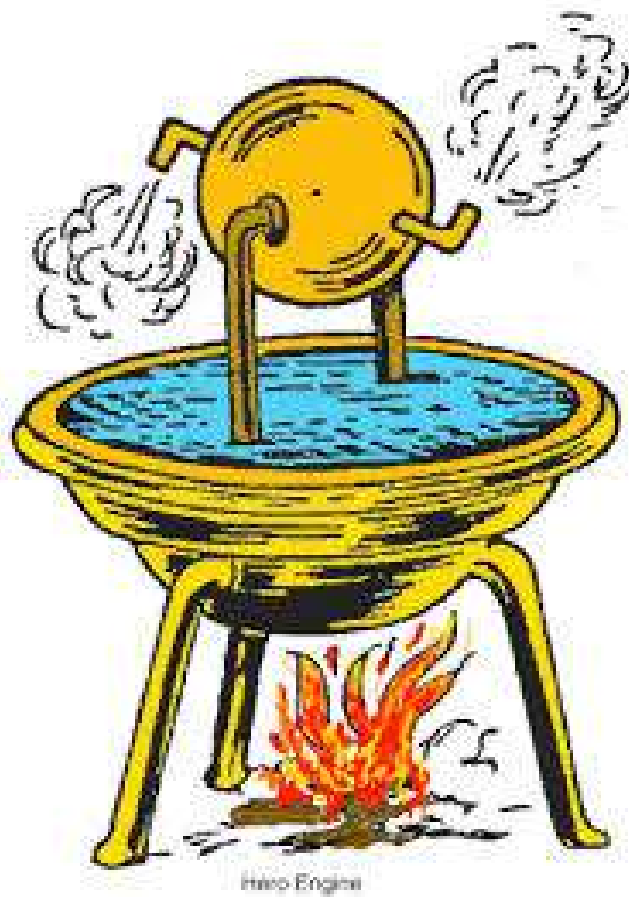
Figure 11.1: A jet-driven steam engine invented by Hero of Alexandria in the 1st century A.D..
