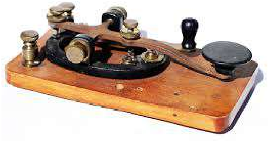
Figure 6.6: An early telegraph key
