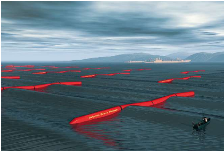
Figure 2.10: The Pelamis wave energy transformer floats on the ocean like a giant sea snake. It consists of several segments which move against each other and build up hydraulic pressure. This in turn drives a turbine. A new Pelamis generation is currently under construction.
