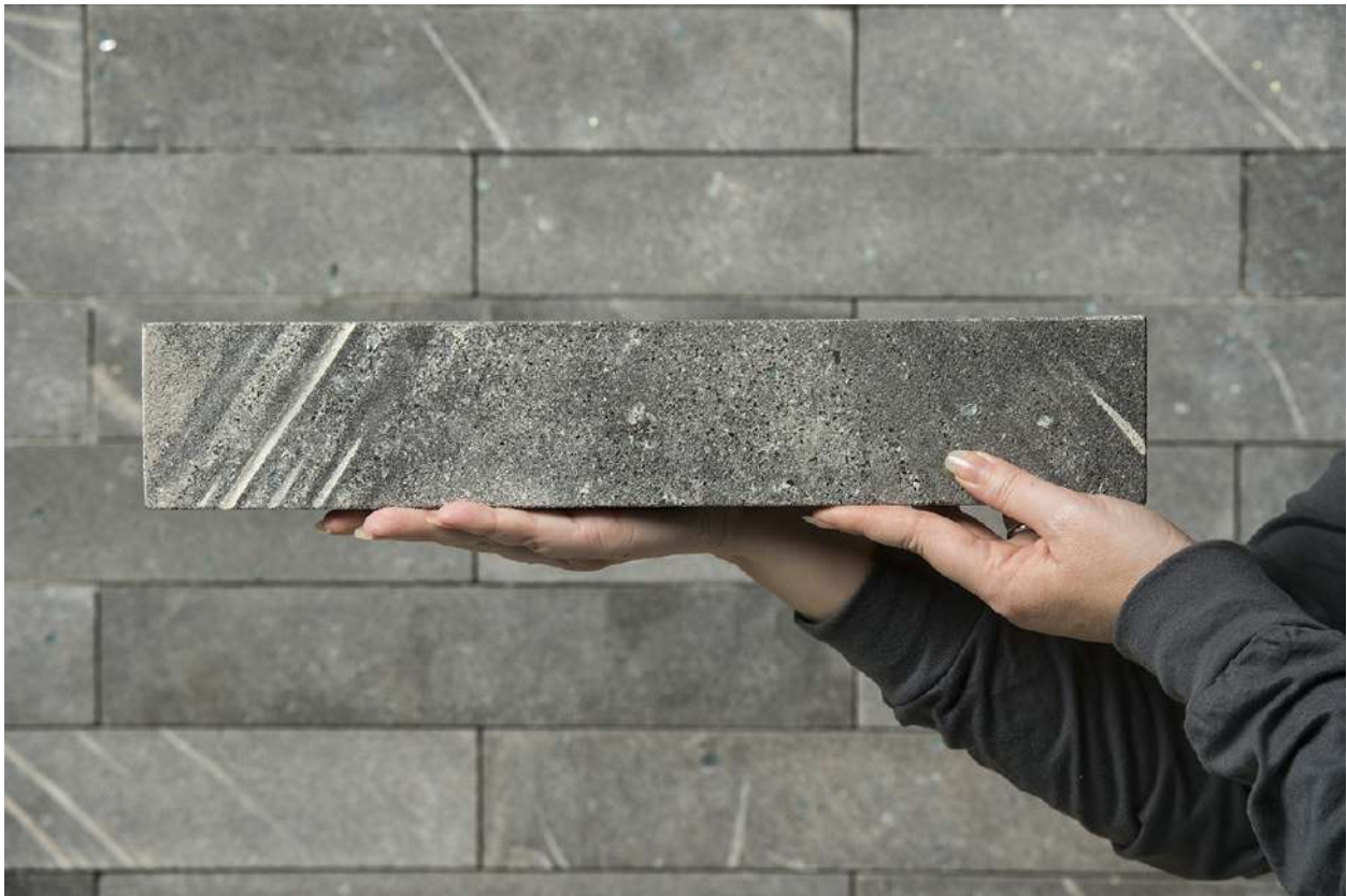
Figure 3.21: BioMason uses bacteria to grow cement bricks which it says can sequester carbon. Credit: bioMASON, Inc..
