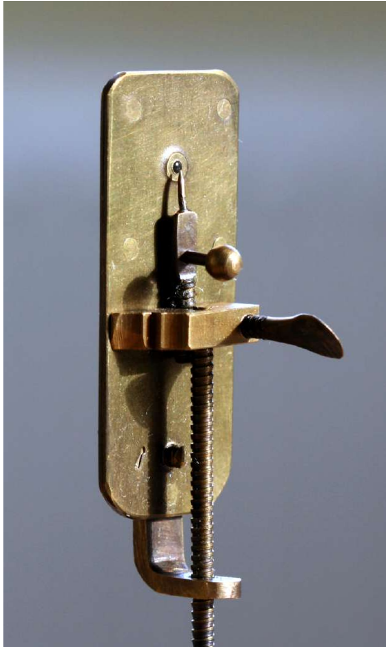
Figure 3.3: A replica of a microscope by van Leeuwenhoek. The single-lens microscopes of van Leeuwenhoek were relatively small devices, the largest being about 5 cm long. They are used by placing the lens very close in front of the eye, while looking in the direction of the sun. The other side of the microscope had a pin, where the sample was attached in order to stay close to the lens. There were also three screws to move the pin and the sample along three axes: one axis to change the focus, and the two other axes to navigate through the sample.
