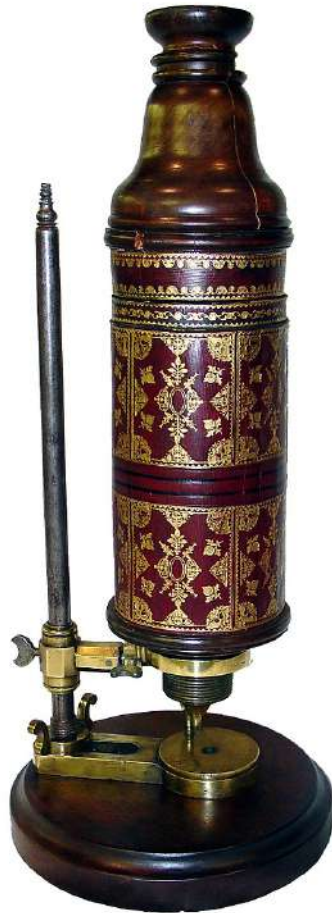
Figure 3.4: Microscope manufactured by Christopher White of London for Robert Hooke. Hooke is believed to have used this microscope for the observations that formed the basis of Micrographia .
